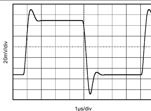
Figure 6-20. Large-Signal Step Response
