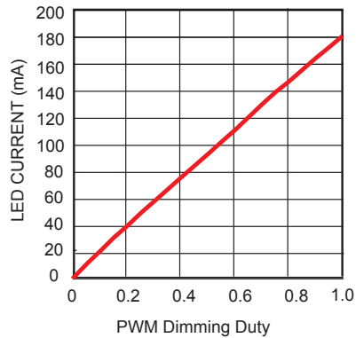
LED Current vs. PWM Dimming Duty
